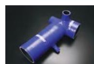
ASHK220 BRZ induction hose for stock air box Inner Steel ring to reinforce hose strength ( 1pc )
